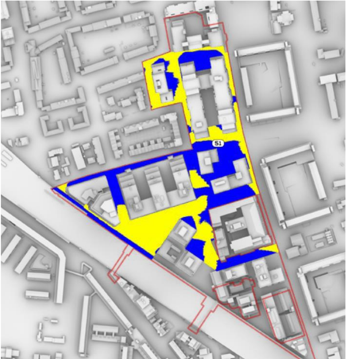
Overshadowing diagram, yellow areas receive at least 2 hours of sun on 21 st March, blue areas do not
