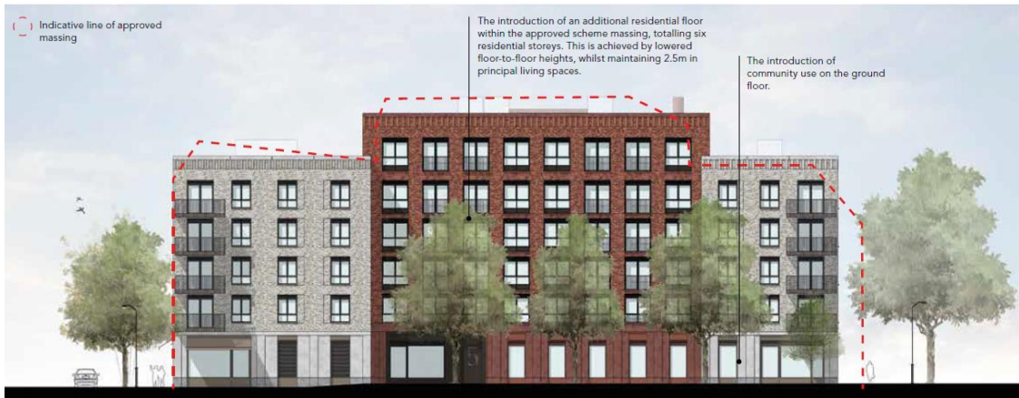
Proposed eastern elevation of block 5
